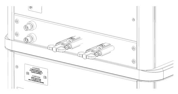
The high pressure "E" size cylinder yoke/regulator assemblies, pipeline inlets, and piping manifold are all mounted on the gas tray, which is bolted to the rear of the machine. This tray can be completely removed for ease of servicing.
