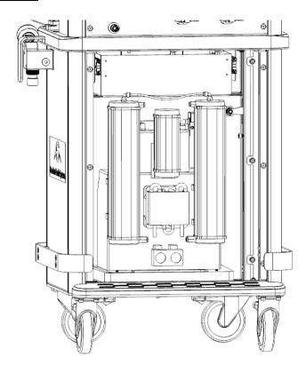
The oxygen concentrator is mounted onto the base of the UAM and is accessed through the rear cover or front panel. The concentrator is designed for easy removal for servicing with connectors for gas, electricity and the circuit boards being quick release. Four nuts underneath the base hold the concentrator in position.
