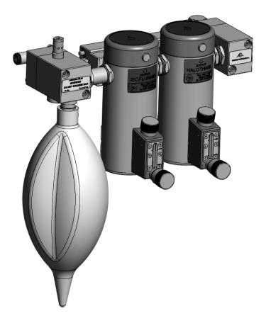
The UAM is fitted with a dual-position vaporizer backbar suitable for a drawover vaporizer. The connections between machine and vaporizer are made with parallel fittings to prevent jamming and potential damage during vaporizer removal.
