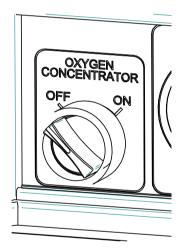
The machine on/off switch is mounted on the left hand side of the gauge panel and is protected by a shroud to prevent inadvertent turning off. This switch turns the oxygen concentrator on. The switch allows pneumatic power to the anesthetic machine and flowmeters.
