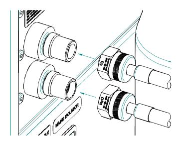
The NIST pipeline inlets are mounted on the rear left hand side of the machine and are marked for gas identification. Each inlet includes a non-return valve and contents gauge connection, with a filter in the manifold block to prevent system contamination with dust.
