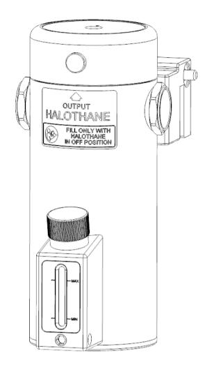
The machine is fitted with a draw over vaporizer with a pour filler. The vaporizer is available for Halothane, Isoflurane or Sevoflurane anesthetic agents. Filling level is indicated by a flat glass indicator where overfill beyond the maximum fill level is also indicated. Filling must take place only when the vaporizer is attached to the machine and when the machine is on a level surface.
