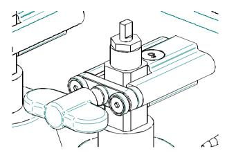
The UAM can be fitted with a maximum of 2 yokes – 1 oxygen and 1 nitrous oxide. Each yoke is pin indexed to prevent connection of the wrong cylinder and has a colour coded gas identification label.
