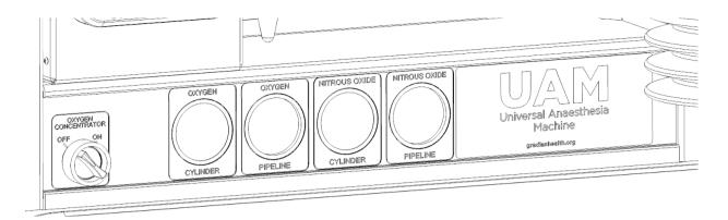
The cylinder and pipeline contents gauges are mounted below the flowmeter bank in an aluminium extrusion with a Perspex cover set into the extrusion.
