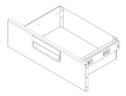
A metal drawer unit is mounted under the work surface. The drawer is removable for cleaning by fully opening and then pressing the toggle lever on the end of each slide to remove the drawer.
