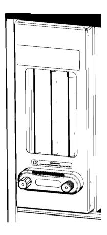
The flowmeter bank is available as a 2 gas oxygen and nitrous oxide option only.
