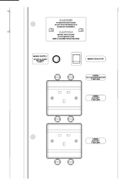
Mains power supply is 220 - 240 volts 50 – 60 Hz the power lead is service personnel replaceable and is 1.25 mm - 13 Amp, 4 metres long and is fitted with a UK style 3-pin plug fused for 13 amps. An isolator switch is fitted which is illuminated when on and isolates incoming power to the oxygen concentrator and the two auxiliary power sockets.
