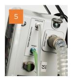
5) The pressure and control lines are attached correctly, with the pressure line (green) connecting the bottom of the valve to the blue port on the CCV marked PATIENT AIRWAY and the control line (clear) connecting the top of the valve to the silver port on the CCV marked EXHALATION VALVE. Connecting these tubes improperly will prevent the ventilator from functioning and will cause errors.
