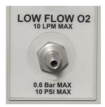
0.7 Bar (10 psi) and for flows of 10 LPM or less. Any higher pressure or flow could lead to the hose being blown off of the barb.
