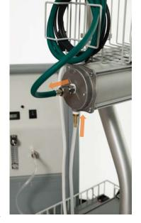
facing the machine): a hose barb inlet threaded fitting outlet to be connected to the CCV's DISS port via the provided hose. When not in use, both ports should be plugged, the inlet by leaving the provided flexible silicone hose attached for quick access, and the outlet by the provided red plastic cap. Keeping the ports plugged will prevent any cleaning fluid from entering the reservoir, which would then pose a danger to the patient as fumes or vapors could be inhaled.
