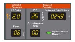
**I:E Ratio** is the ratio of inspiration time to expiration time. The ratio is always expressed as 1:Y where Y is the expiration value. Thus, when the illuminated display shows 2.0, the I:E ratio is 1:2, and the expiration time is twice as long as the inspiration time. The ratio is determined by the clinician's choice of inspiration time and respiratory rate.
