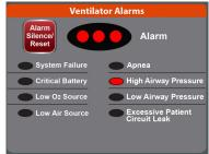
To mute the audible alarm for 110 seconds, press the Alarm Silence/Reset button. The alarm lights will stay on. Any new alarm conditions will also trigger the audible alarm.
