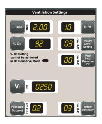
\*\*O₂ is a **setting, not a measured value**, and may be programmed to deliver between 21% (room air) and 100% oxygen. The purpose of the \*\*O₂ setting is to mix gas from the oxygen source with air from the compressed air fitting or from room air. The \*\*O₂ setting tells the CCV what mix of oxygen and air to use. It does not tell what the FiO₂ is, just what the CCV is using as a target value.
