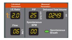
**I:E Ratio** is the ratio of inspiration time to expiration time. The ratio is always expressed as 1:Y where Y is the expiration value. Thus, when the illuminated display shows 2.0, the I:E ratio is 1:2, and the expiration time is twice as long as the inspiration time. The ratio is determined by the clinician's choice of inspiration time and respiratory rate.
